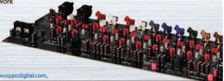
OPPO BDP-95 Analog Audio Board Featuring Two ESS ES9018 SABRE 32 Reference Audio DAC Chips
